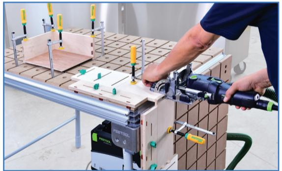
Build a gridded dovetail work table with horizontal and vertical work surfaces to make accurate, repeatable 90° joinery and build drawers in less than half the time.
