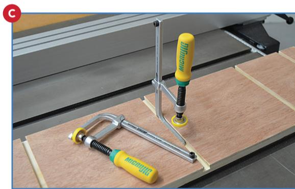
3. The head of the MATCHFIT Dovetail Clamp is forged 1/2" wide with 14° angles on each side so it slides easily within a 1/2"x14°x3/8" deep dovetail slot that you cut wherever needed. **C**
