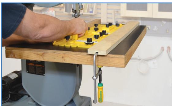
Custom fences, like this one on a bandsaw auxiliary table, can be made to order in minutes. This makes the most of your shop machines and time.
