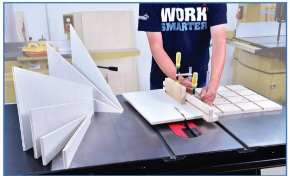
Build a 360° dovetail table saw sled. The fence can be locked from 0° to 360° in any groove. Cut panels at any angle or width that fit on the sled. A ZEROPLAY Miter Bar or equivalent should be installed on the 360° dovetail sled.
